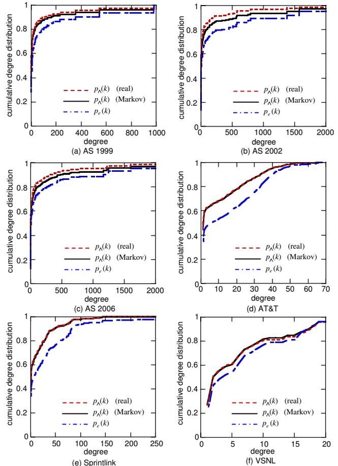
Fig. 5. Degree distribution under wedge-based sampling
