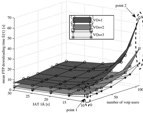
Fig. 1. Multiplexing gain from virtualization represented by decreasing FTP downloading time because of spectrum sharing (simulations)
