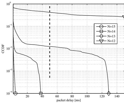
Fig. 6. Validation on resource budget based on 20 ms estimation: packet delay performance of 200 VoIP calls,  $N$ : number of PRBs reserved
