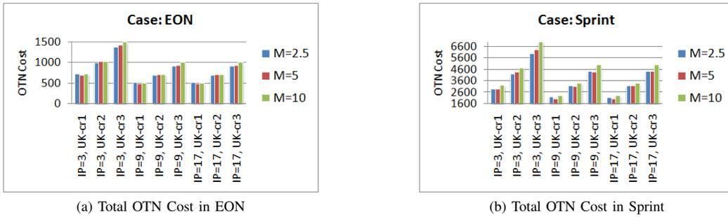
Fig. 8. Total OTN Cost of Different  $M$  and  $U_k$ .
