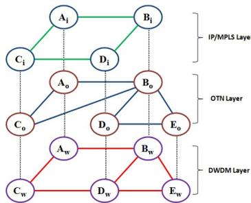
Fig. 1. IP/MPLS over OTN over DWDM Network
